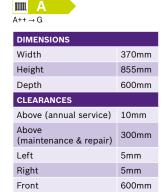
The appliance is suitable for an under-worktop installation providing that the worktop above the boiler (min. 10mm clearance) is removable for maintenance and repair.
